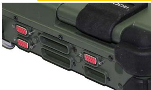
Picture 1: Sealed and opened interfaces of a SDIP 27 Level A Rocky®
